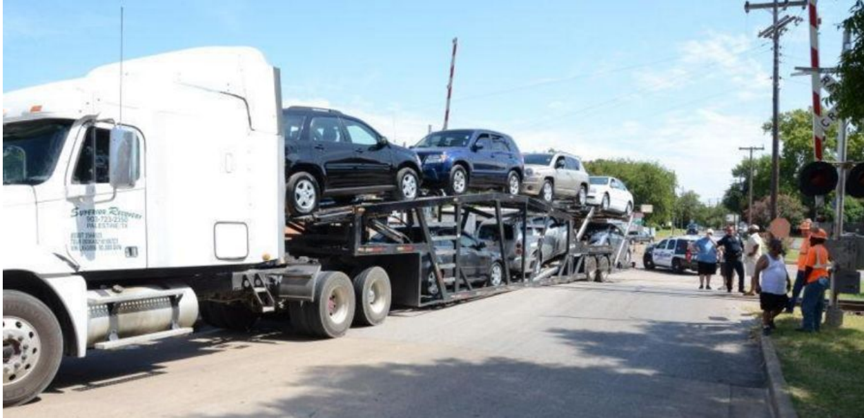
Figure 31. Auto-Transport Trailer High-Centered on Tracks in Waxahachie, Texas [28]
