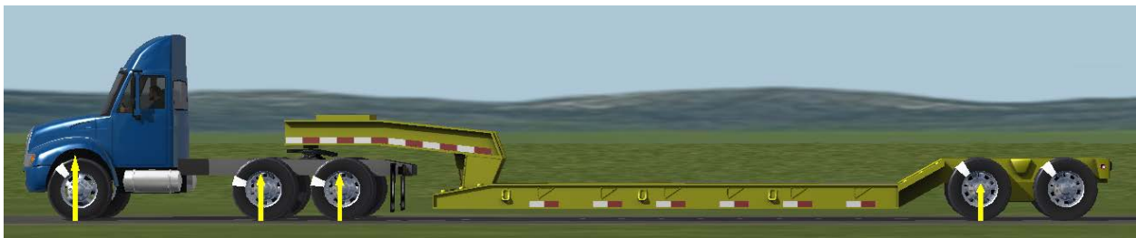
Figure 135. TruckSim Tractor with a Lowboy Trailer Model
