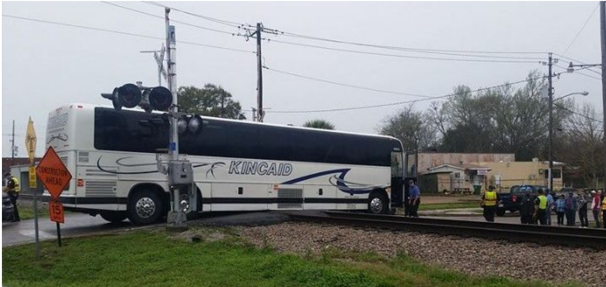
Figure 28. Charter Bus High-Centered at Main Street Crossing in Biloxi, Mississippi on March 12, 2016 [41]
