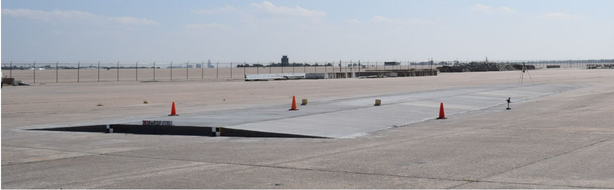
Figure 39. Speed Table for Test Nos. UTCRS-1 through UTCRS-4
