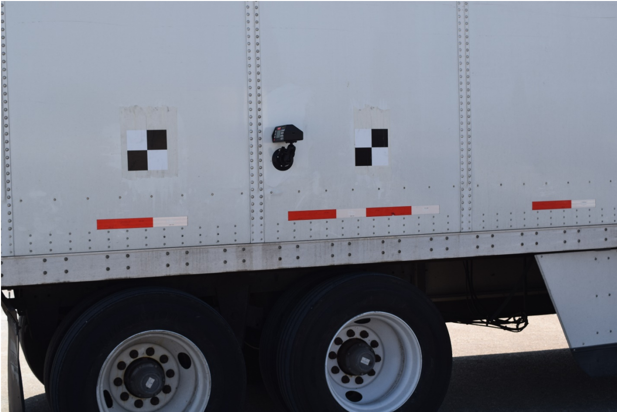
Figure 49. VC4000 Accelerometer Mounted on Trailer
