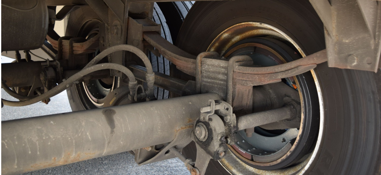
Figure 47. Leaf Springs on the Right Rear Wheel of the Crete Carrier Trailer
