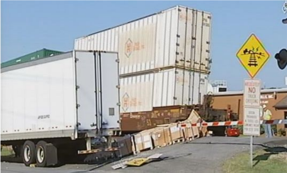
Figure 36. Low Ground Clearance Warning Sign Posted at Crossing [32]
