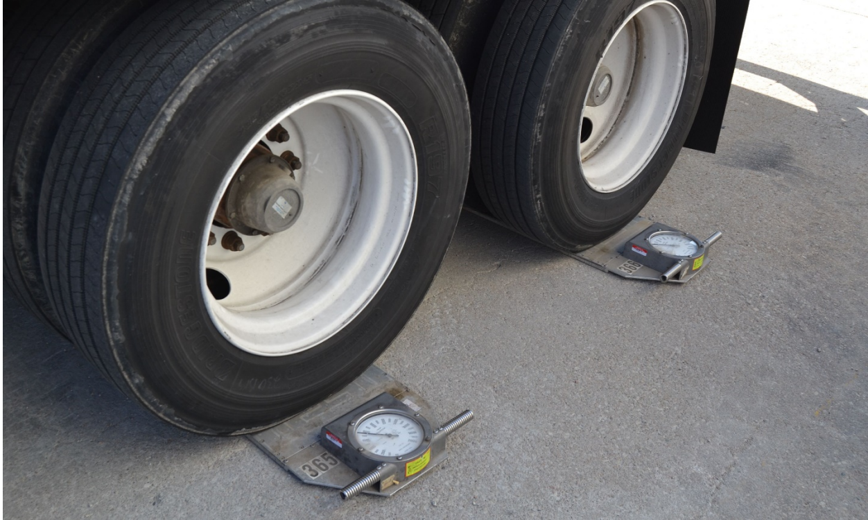
Figure 43. Portable Heavy Duty Truck Scales Weighing the Crete Carrier Tractor-Trailer
