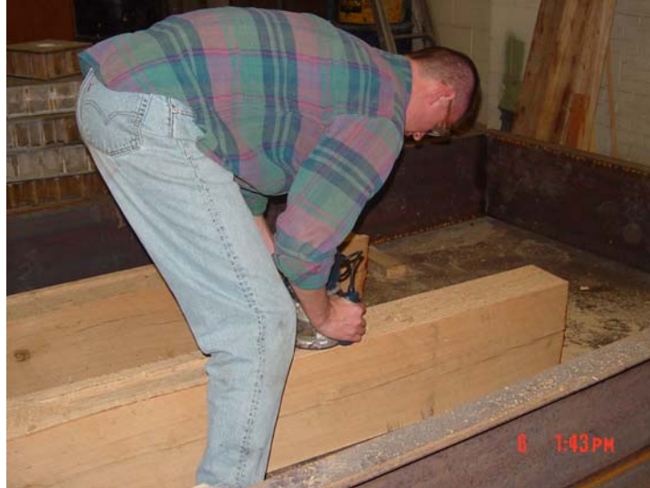
Figure 17. Photo. Routing of test specimen.
