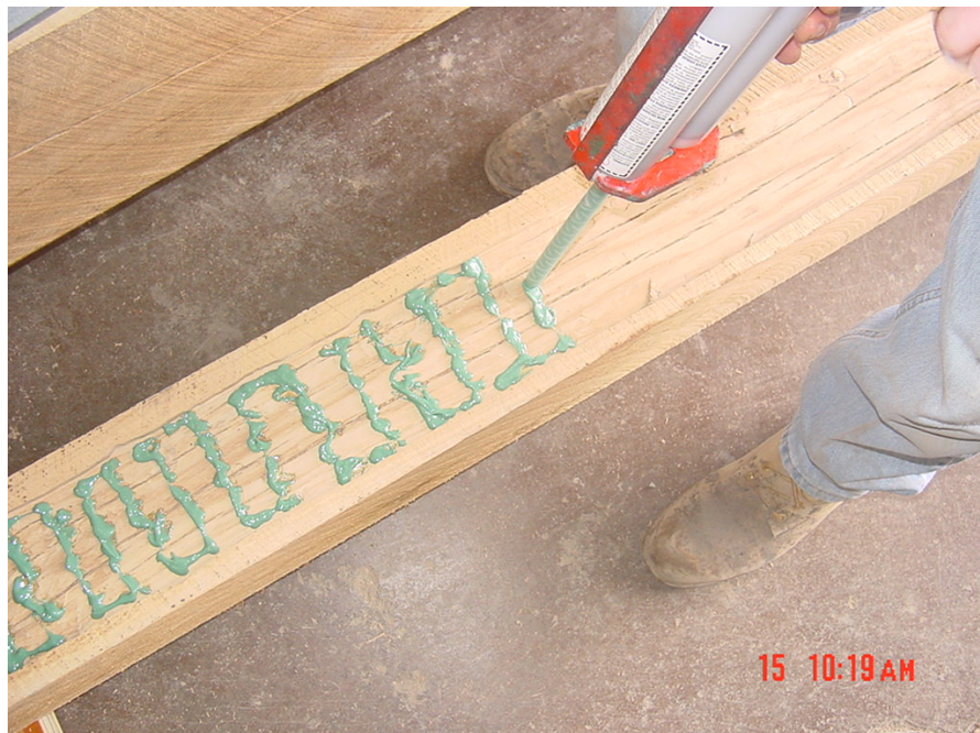
Figure 18. Photo. Applying adhesive on test member.
