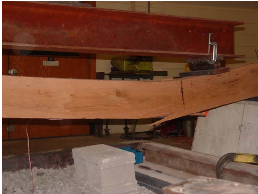
Figure 74. Photo. Shear failure of B1 directly under loading point.
