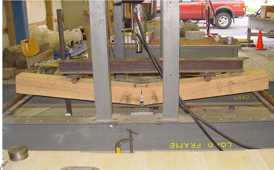
Figure 56. Photo. Specimen after testing.
