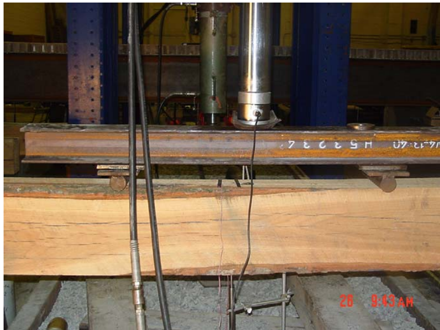
Figure 38. Photo. Side view of reinforced specimen.
