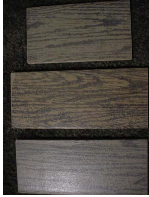
Figure 40. Photo. GFRP with veil.
