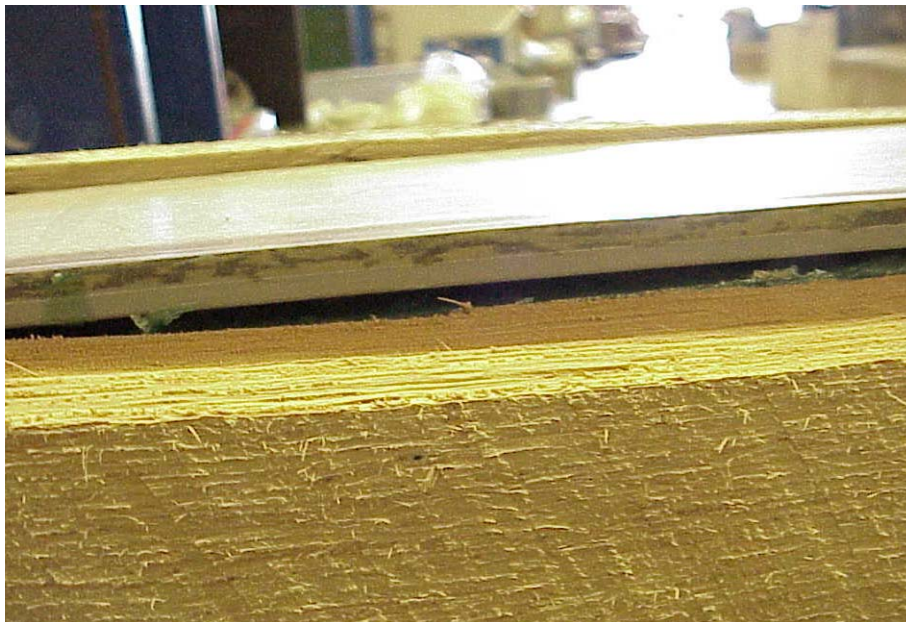
Figure 62. Photo. Bond failure of LB-8.
