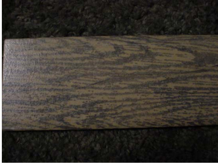
Figure 41. Photo. GFRP with veil.
