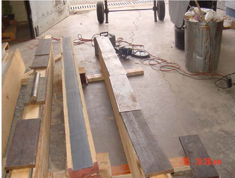
Figure 19. Photo. Steel plates used as weights on test specimen.
