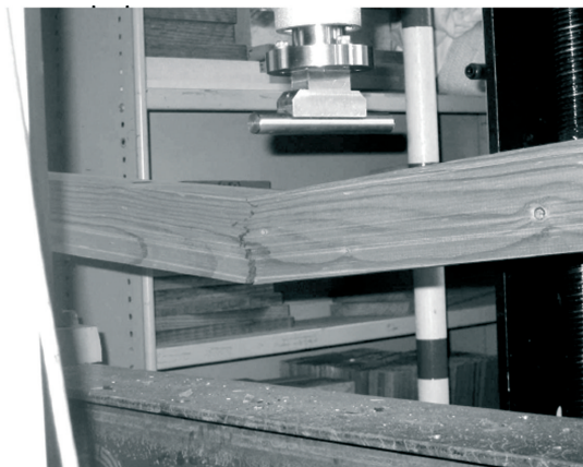
Fig. 7b The typical fracture of a completely treated Norway spruce specimen after a bending test
