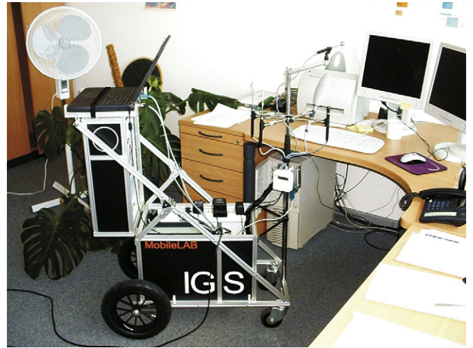
Fig. 3. The applied mobile unit measuring a user's comfort envelope.
