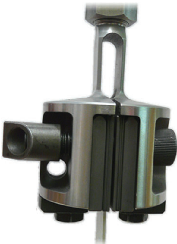
Figure 4 Grips system used at the moment, which belong to a resonant testing machine.
