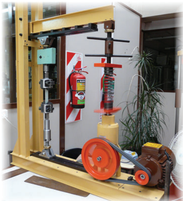
Figure 7 Photograph of the built machine working with only one spring.
