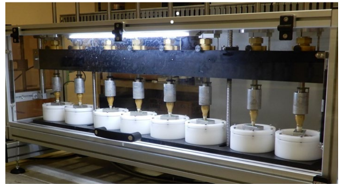
Fig. 5. Artificial aging of specimens after transfer to a chewing simulator. During artificial aging, both insertion (with 53 N of force magnitude) and removal of the crowns took place with a crosshead speed of 30 mm/s.
