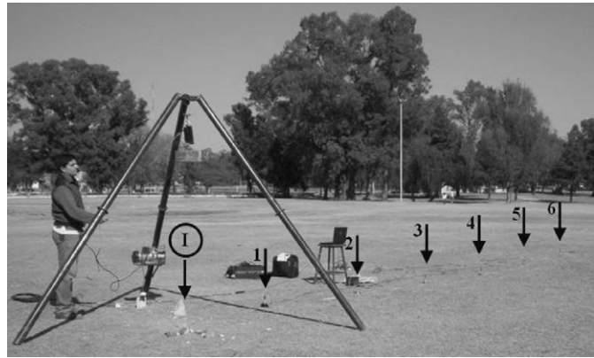
Fig. 7. Application of impulsive load and transducers layout for Case 1.
