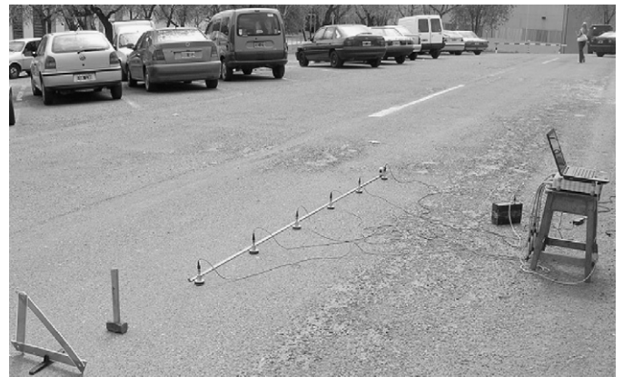
Fig. 12. Application of impulsive load and transducers layout for Case 2.
