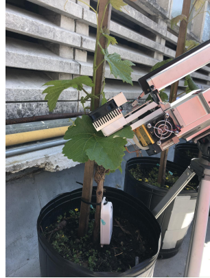
Figure 1. Potted Grapevine cv. Tannat with IRGA at the leaf and electrodes
