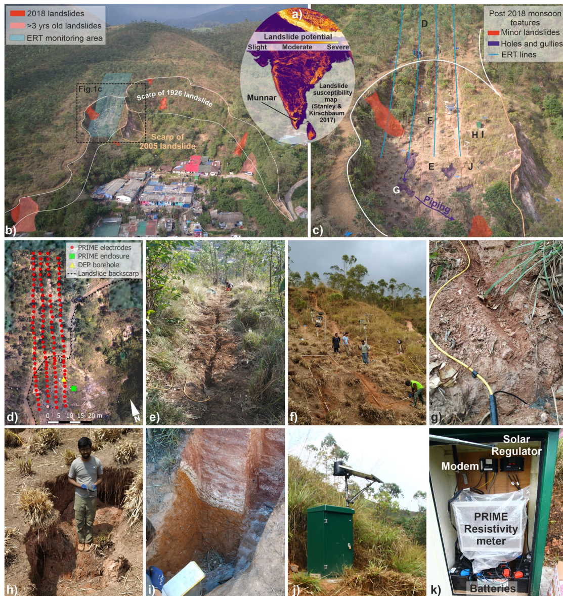
Fig. 1 a Location of Munnar overlaid on the Indian portion of the landslide susceptibility map by Stanley and Kirschbaum (2017) (image: NASA). b General overview of the Amrita-LEWS site, as of February 2019, showing the remnants of past landslide events. c Aerial view on the ERT monitoring area highlighting the landslide features and the electrode array. d Map of the deployed ERT monitoring system at the
