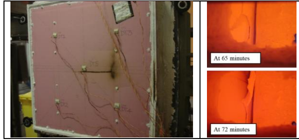
Fig. 9 | Unexposed surface of Specimen 3 after fire exposure and time instants where fall-off of the exposed gypsum plasterboard occurred.
