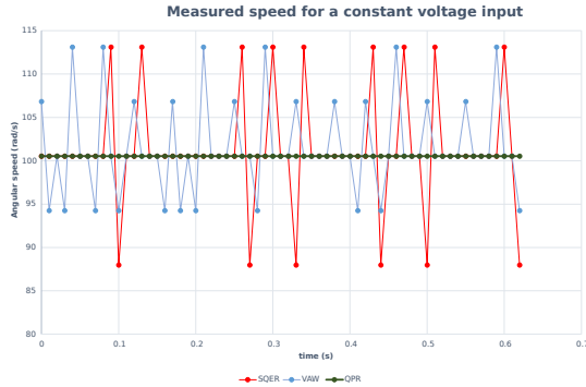
Fig. 9: Constant speed. The red line is the standard reading (SQER), the blue is the VAW and the dark green is the QPR (including the VAW).
