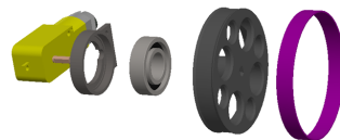
Fig. 3: Exploded view of the wheel connection.
