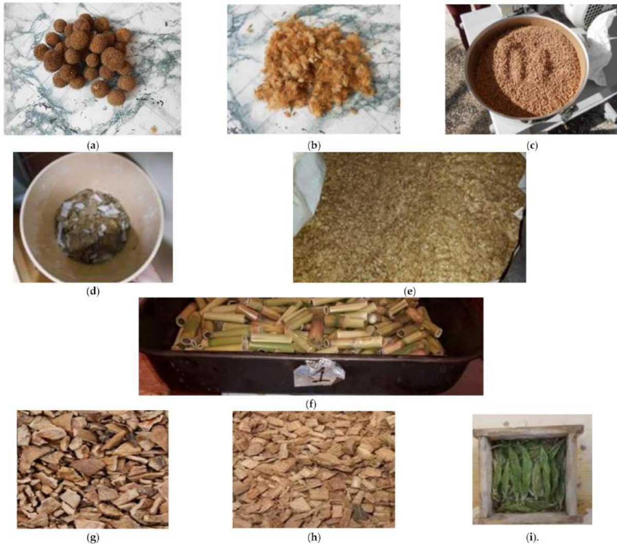
Figure 2. Natural/waste materials: (a) Desiccated platanus acerifolia fruits; (b) Smashed desiccated platanus acerifolia fruits; (c) Triturated cork plugs; (d) Water-soaked cardboard; (e) Coffee parchment skin; (f); Chopped cane stalks (g) Almond and nut shells; (h) Coconut shells; (i) Bean and pea pods.
