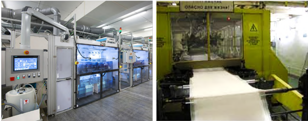
Figure 90: Example of electrospinning system on industrial scale. Nanospider industrial electrospinning technology of Elmarco ( https://www.elmarco.com ; http://electrospintech.com/mass-production.html#.Y00hzC0QNAY ).
