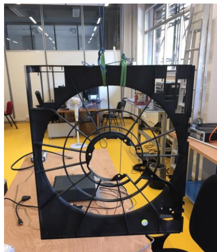
Figure 4.5. Casing elastically suspended to simulate the free-free condition for modal testing.
