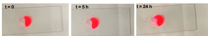
Figure 4. Pictures of the cut halves of the gel of DBS in [bmpyrr][NTf 2 ] (3 wt %) taken at different times.
