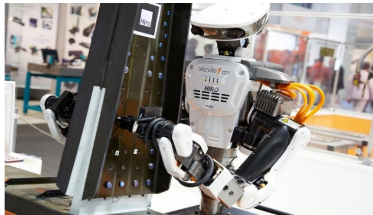
Figure 2. Robot Kawada Nextage Open of TecNALIA [13].
