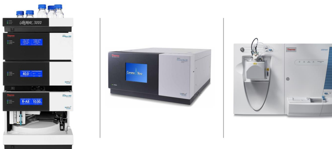
Figure 6: Thermo-Fisher (1) UltiMate 3000 UHPLC system, (2) Corona Veo RS CAD detector and (3) LCQ Fleet Ion trap Mass Spectrometer used for the GNP characterization.
