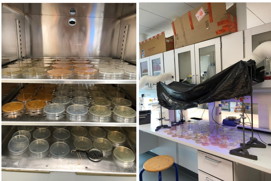
Figure 3. Pictures of plates growing when initially cultured both under the set ups for C1 in the left (darkness and 28 °C) and under C2 in the right (UV light and room temperature). Pictures taken in the AAU laboratories (Esbjerg).
