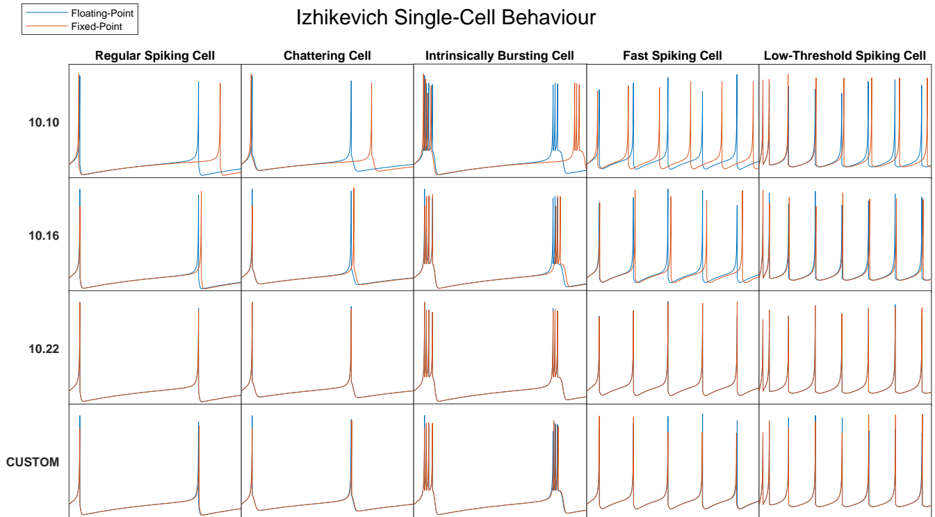
FIGURE 8. Fixed- and floating-point Izhikevich single-cell membrane potential superimposition at the varying of the fixed-point data width. The waveforms have been captured within a time window of 200 ms. On the left is indicated the fixed-point data format. Each column depicts a different kind of neuron, from left to right regular spiking, chattering, intrinsically bursting, fast-spiking, and low-threshold spiking cells.
