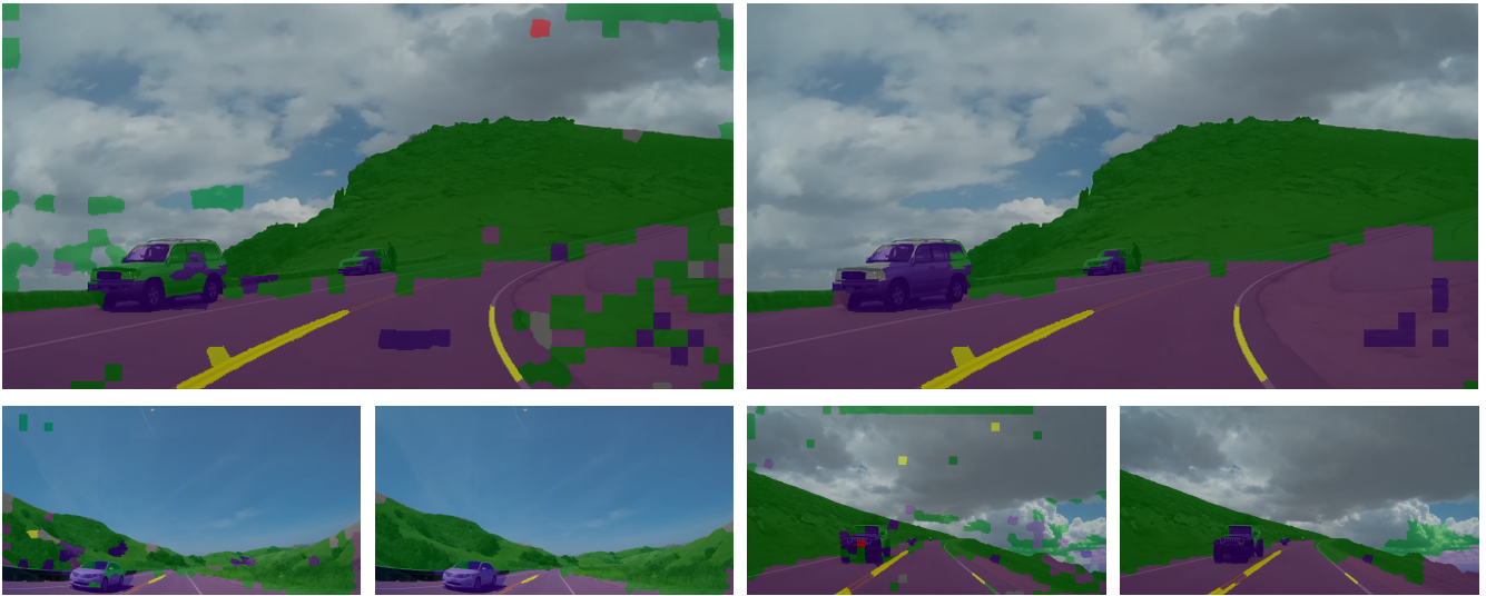
Figure 4: Qualitative comparison between independent logistic regression classification (left images) and structured prediction (right images), using the same classes as in Fig. 3. The top two images feature two vehicles, the bottom left images one vehicle (black colored regions represent unknown labels), and the bottom right images two vehicles. The logistic regression classifier leads to spurious labels, which are filtered out by the structured predictor. The image legend is equal to the legend in Figure 3.
