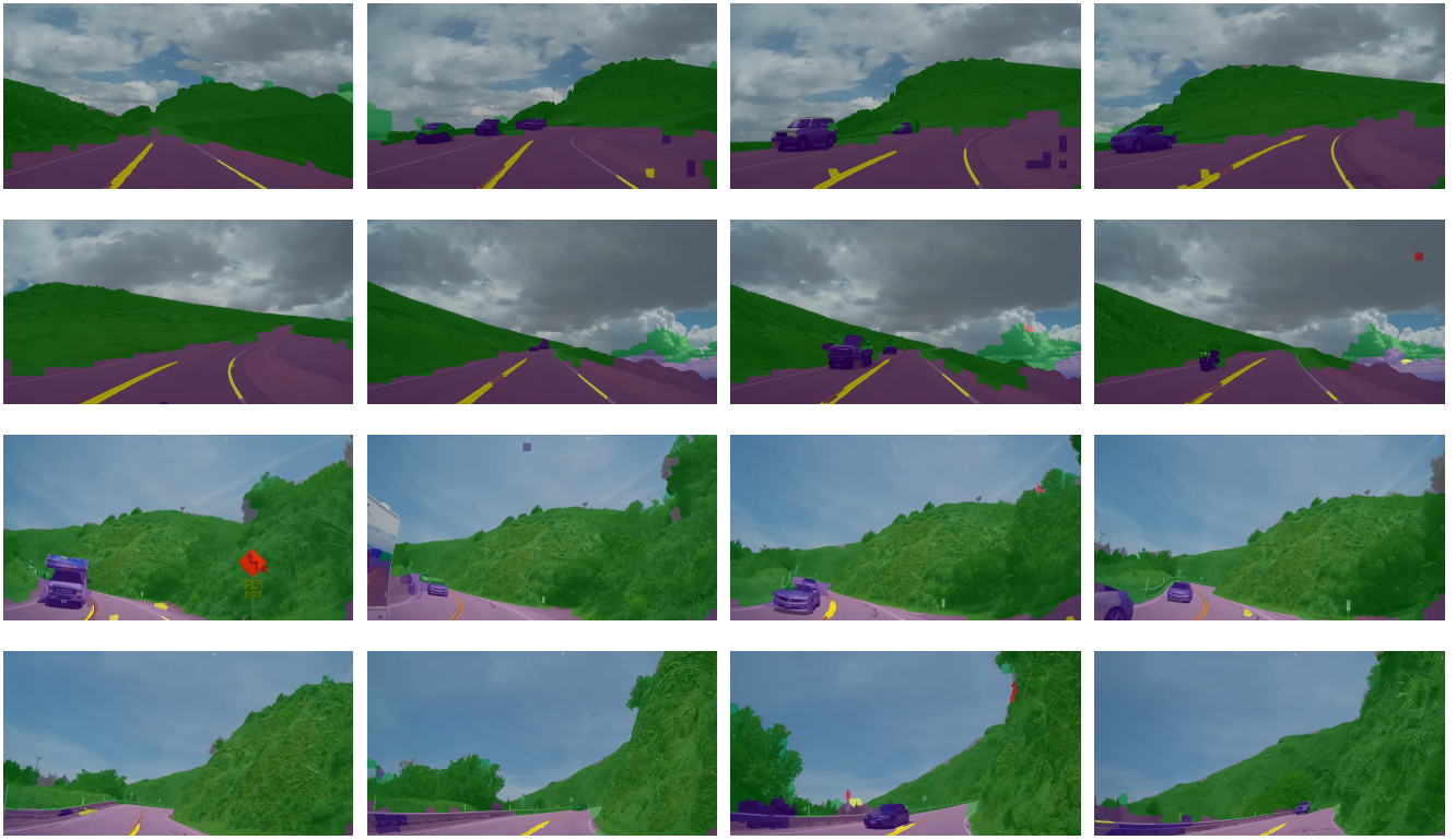
Figure 3: Unseen samples from two dashboard camera videos (time flows from left to right, top to bottom) segmented. Legend: road (light purple/pink), vehicle (dark purple), vegetation (green), sky (gray), road marking (yellow), and road sign (red).
