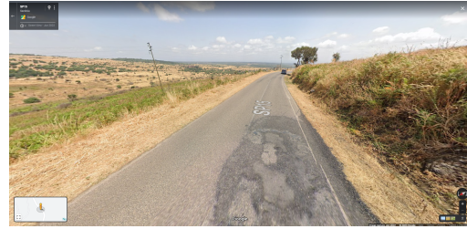
Figure 6.2. Google Street View 2022 capture [59] showing a patch of residue from the car fire still present on the Provincial Road 15. Using the picture on the left, it was possible to find the precise coordinates of the car, and therefore the likely ignition point. Note the electrical pole on the left.
