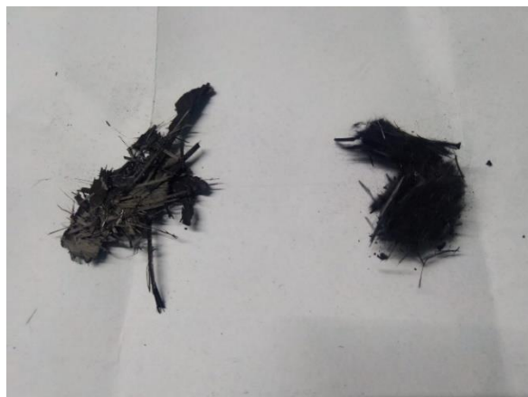
Figure 6.21 Resin-bonded CF (on the left) and non-bonded CF (on the right)
