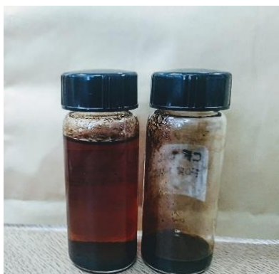
Figure 6.22 Aqueous phase (on the left) and organics (on the right) of CF
