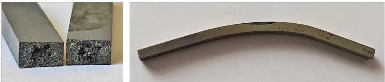
Figure 11. Macrographs showing a shrinkage cavity (left) on a fracture surface and a bent specimen (right) after mechanical test at 950 °C.
