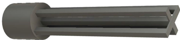
Figure 1. Drawing of the wax pattern used to produce the specimens.
