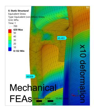
**FIGURE 3.** (left) Temperature map from the FEA thermal analysis. (right) Stress and deformation (magnified *times* 10) from the FEA mechanical analysis.
