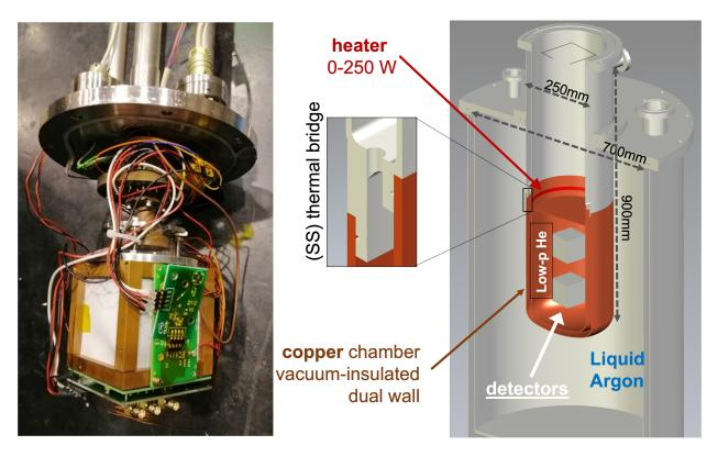
**FIGURE 2.** (left) Detector module equipped with one SiPM array and mounted on a temporary cryostat support. (right) Cryostat CAD model with detail on the thermal bridge.
