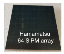
**FIGURE 4.** (left) Custom FBK 24-devices array. (center) Croygenic amplifier designed for FBK array. (right) Hamamatsu commercial 64-devices array. All sensitive areas are  $50 \times 50 \text{ mm}^2$ .
