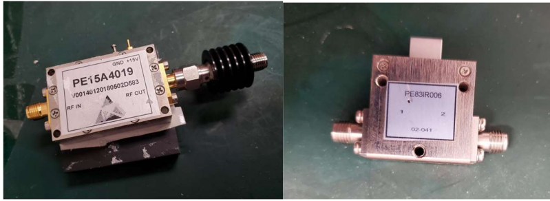
Figure 2.17 Medium power GaAs amplifier PE15A4019 is used in the transmitter network (left) RF isolator used to prevent back reflections (right)
