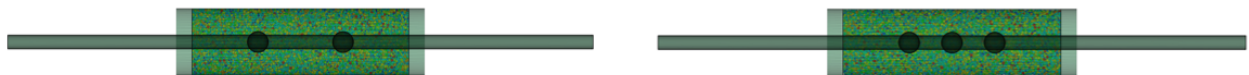
Figure 5.33. Different configurations of the sand damper tested numerically in DEM simulations: Left: Damper with two metal spheres appended on the piston rod; Right: Damper with three metal spheres.
