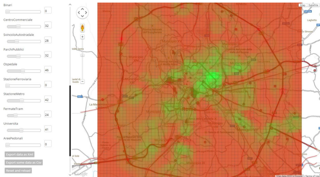
Figure 3: InViTo interfaces: setting weights and output accessibility maps (red colour = areas with lower values of accessibility; green colour = areas with higher values of accessibility).
