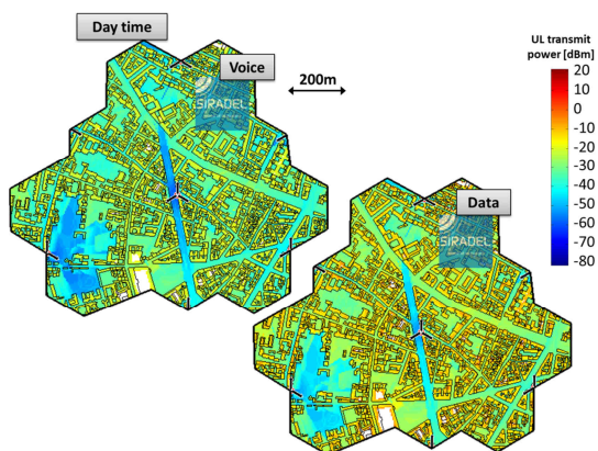
Figure 3: Tx power (dBm) calculated indoor at ground floor and outdoor during the day for voice and data traffic
