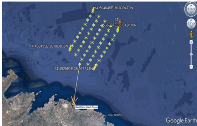
Figure 6. Satellite imagery of the wind farm showing the location of the 50 wind turbines with respect to the coastal lidar station (©Google Maps 2019).
