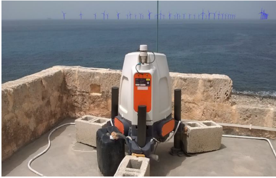
Figure 5. View of the wind farm rendered onto an image of the area and also showing the lidar unit.
