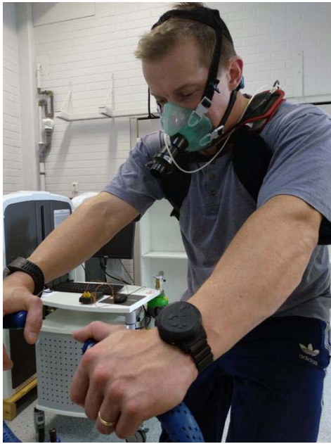
Fig. 2. Experimental setup: the subject is wearing a custom-made bracelet equipped with HF and temperature sensors on his left hand. A reference EE value was obtained using a spirometry calorimeter; furthermore, the subject's heart rate was monitored using an ECG chest strap.
