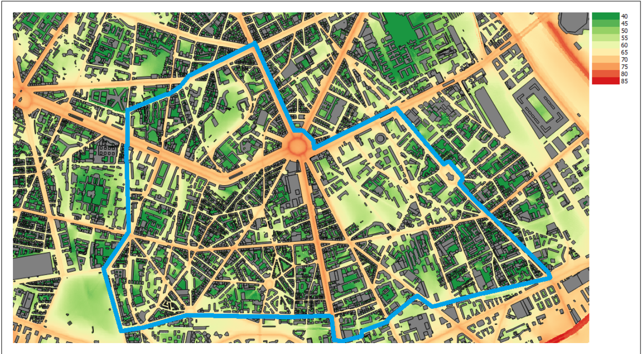
Figure 2. Static noise map (distribution of L_{den} ) of the study area. The boundary of the study area is highlighted in blue.
