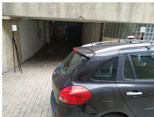
Figure 7. The starting point of the measurement lap at the entrance of the garage and the location of the employed GNSS antenna and UWB tag on the roof of the car.
