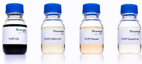
Fig. 7. TCR-oil, hydrogenated TCR-oil, TCR-diesel and TCR-gasoline.
