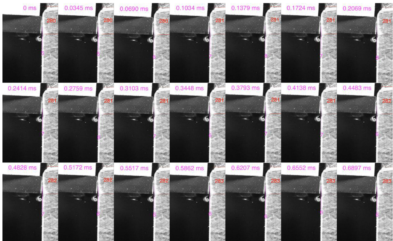
Fig. 8 Successive screenshots that contain the pixel value as the criterion to indicate the behavior change in the cutter for Spike 7 in the cutting process with v=6 m/min and FOA=90^\circ .
