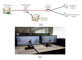
Figure 3: The PoC is composed by a video server, an OpenFlow switch connected to an OpenFlow controller, a layer 2 switch and two video clients.
