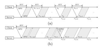
Figure 1: An example live video scenario for HTTP/1.1 (a) and HTTP/2 (b), where the client requests m available segments to ramp up the buffer. Note that  $r_i$  denotes the release of segment i at server side,  $s_i$  its request/download by the client and  $q_j$  indicates that the server should change the quality of pushed segments to j.
