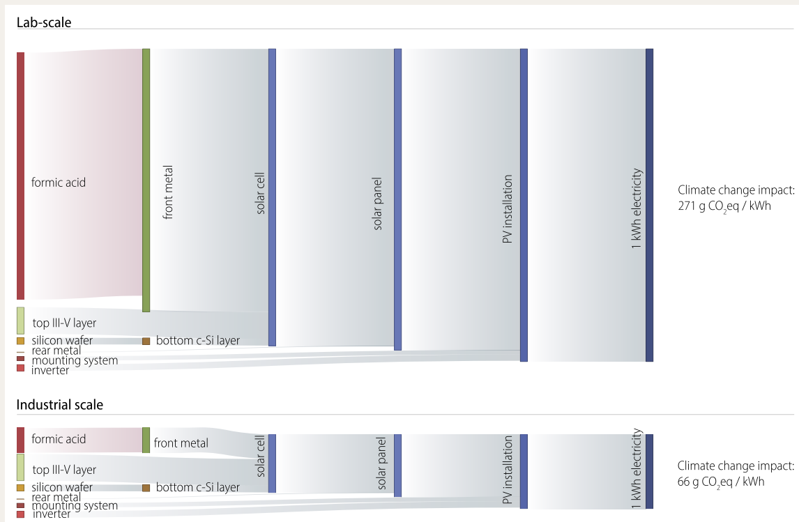
Figure 3 | Process contributions to climate change impacts of III-V/Si panels with lab-scale (top) and industrial-scale (bottom) sintering of front contacts (left) and upscaled sintering (right) (credits: Mirella El Gemayel).
