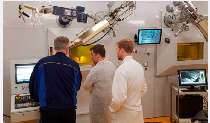
Figure 3: An important milestone was the successful fully-remote recovery of a test specimen series from the surveillance package of one of the domestic plant operators. The in-cell CNC machining station positioned inside the heavily-shielded reception hot cell, made by Finnish company Metecno Oy, was a key device in the precise operation.
