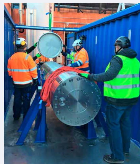
Figure 2: The A-type certified radioactive materials transportation cask VTT procured with investment aid was custom-designed with internal cavity dimensions to contain the variety of different surveillance test specimen package designs expected of the reactors existing or being constructed in Finland.
