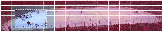
Figure 1: Illustration of the tile-based method. The tile borders are indicated by the white lines. The red areas are not transmitted to the user. The gray areas indicate the pixels that are not displayed on the user side.
