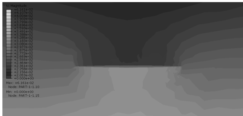
Figure 4. Simulated displacement field around a crack
