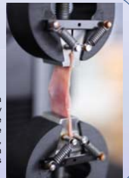
Fig. 1 To analyse the stretch tolerance of the pulmonary vein of pigs, as a prerequisite for using expandable intraluminal ablation devices, pulmonary vein tissue, taken at the level of ostium II, was stretched to various lengths.
