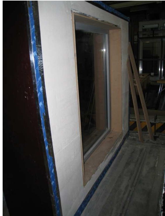
Figure 2a. calibration setup for measuring extraneous air leakage of the setup. Figure 2b. Installation of aluminum window frame and wood reveal.
