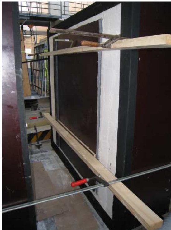
Figure 2a. calibration setup for measuring extraneous air leakage of the setup. Figure 2b. Installation of aluminum window frame and wood reveal.
