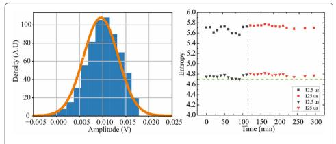
**Figure 8** (a) Histogram of classical noise between peaks for the first 125  $\mu$ s file with the orange line illustrating the Gaussian fit, (b) min entropy values for all 26 files including classical noise (square) and after the removal of the Gaussian noise (triangle)
