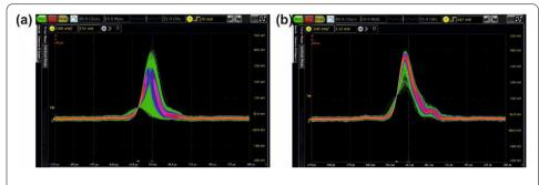
**Figure 3** Amplitude fluctuation of the GS operation (**a**) DC bias near threshold, I = 18 mA, (**b**) DC bias above threshold, I = 33 mA
