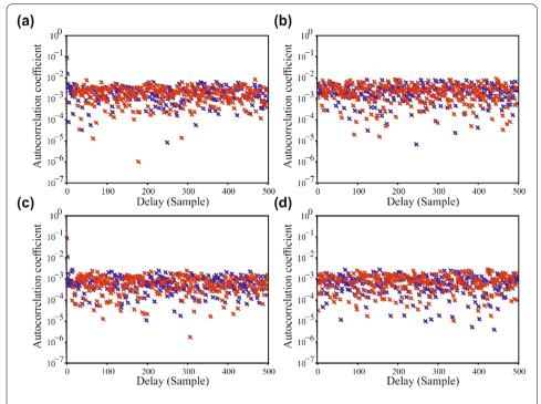
**Figure 10** Autocorrelation coefficient for the last 12.5  $\mu$ s file (a) before and (b) after post-processing with the Toeplitz extractor, (c) Autocorrelation coefficient for the last 125  $\mu$ s file and (d) same file after post-processing with the Toeplitz extractor
