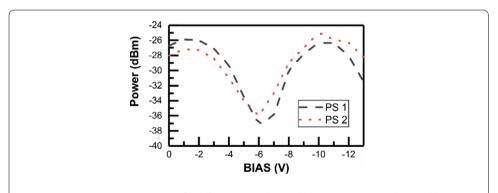
Figure 5 Power measured at output 2 for different BIAS voltage at balanced MZI upper (dash) and lower branch (dot)
