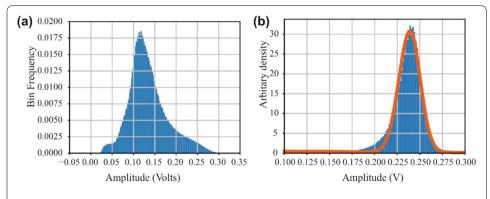
**Figure 6** (a) Bin Frequency vs. peak power in Volts for the first 125  $\mu$ s file at the output of the uMZI, (b) Peak power Intensity variation of GS pulses at output 1, the orange dot line illustrates the corresponding Gaussian distribution fitting
