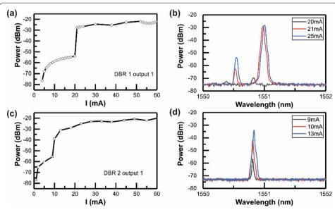
Figure 2 (a) DBR laser 1 P-I curve measured at Output 1 and (b) the spectrum of laser emission near threshold. (c) DBR laser 2 P-curve measured at Output 2 and (d) the spectrum of laser emission near threshold.
