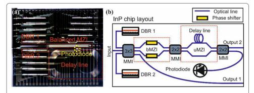
**Figure 1** (a) Top-view photo of the QRNG monolithic integrated InP chip. (b) Chip layout of the QRNG section. DBR: distributed Bragg reflector laser, MMI: Multimode interferometer, u/bMZI: unbalanced/balanced Mach-Zehnder interferometer
