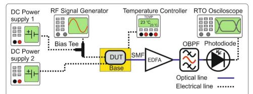
**Figure 4** Experimental set up for the PIC components characterization and QRNG evaluation. DUT: Device Under Test, SMF: Single Mode Fiber, EDFA: Erbium Doped Fiber Amplifier, OBPF: Optical Bandpass Filter, RTO: Real Time Oscilloscope
