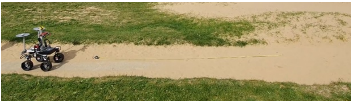
Figure 4.9: Mobile platform used during the experiments driving on concrete for 4 m, then on the sand for 21 m, and again on concrete for 3 m.
