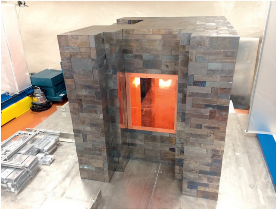
Fig. 3. A photograph of the status of the passive shield assembly, at the time of writing. The outer half of the copper shield, 5-cm-thick and fabricated from commercial copper, forms a box in the center of the shielding. It is surrounded by 45 cm of stacked lead bricks. An inner copper shield fabricated from ultra-pure electroformed copper, veto panels, and polyethylene shield remain to be installed.
