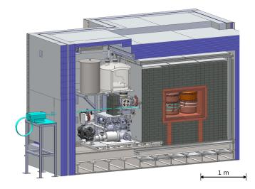
FIG. 2. Cross-sectional drawing of the MAJORANA DEMONSTRA-TOR including, besides the detector cryostats, also cryogenic systems, vacuum hardware, and shielding layers. Copper shielding is shown in brown, lead bricks in dark gray, and the poly shield in purple. Not all muon veto panels are shown for better visibility.
