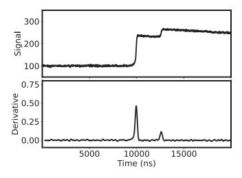
FIG. 4. Top: Two-step wave form (*second* event); Bottom: The first derivative (current) of the wave form. A clear two-step pattern can be observed due to the 53 and 13 keV transitions in sequence.
