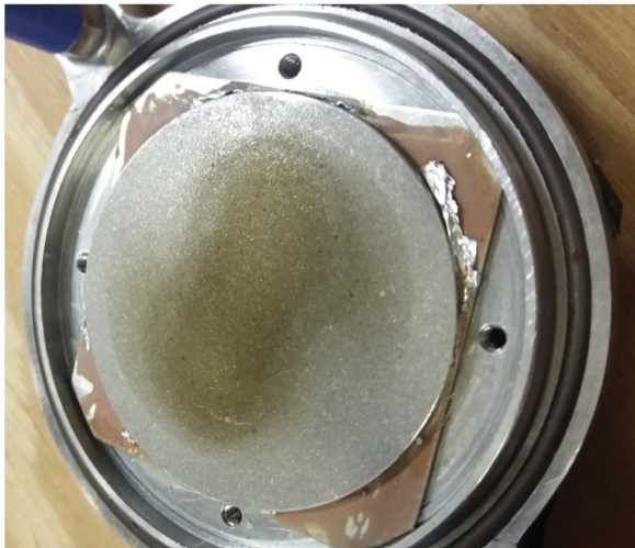
Fig. 7. Sintered titanium target. The round disk is the sintered titanium backing, and the irregular dark spot on the surface is the region with implanted ^{22}\text{Ne} atoms. The brown square around the disk is epoxy affixing it to the square nickel sheet. The target holder is seen behind the target. (For interpretation of the references to color in this figure legend, the reader is referred to the web version of this article.)
