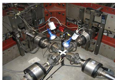
Fig.1. Plane biaxial test device for testing cruciform specimens.
