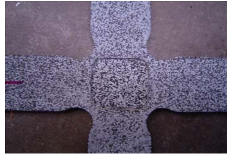
Fig 2b. Applied special speckle pattern.
