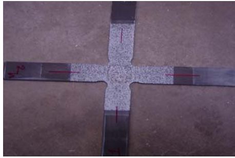
Fig 2a. Cruciform geometry.
