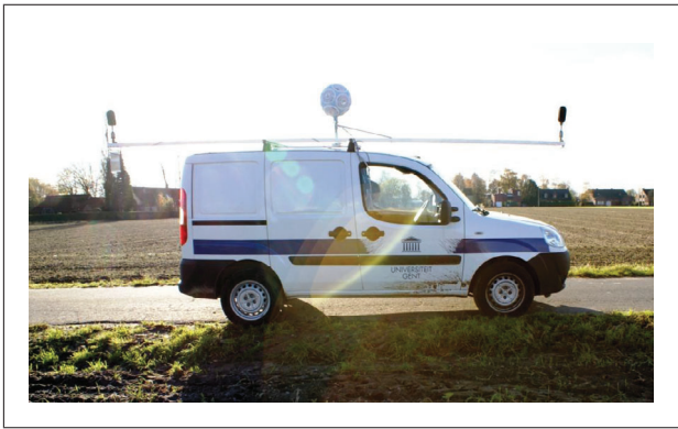
Figure 1. Mobile measurement set-up. An omnidirectional speaker is mounted on the roof of a car. An omnidirectional microphone Type 4189 of Bruël & Kjær is mounted in front and behind the speaker at 2.5\text{ m} distance.
