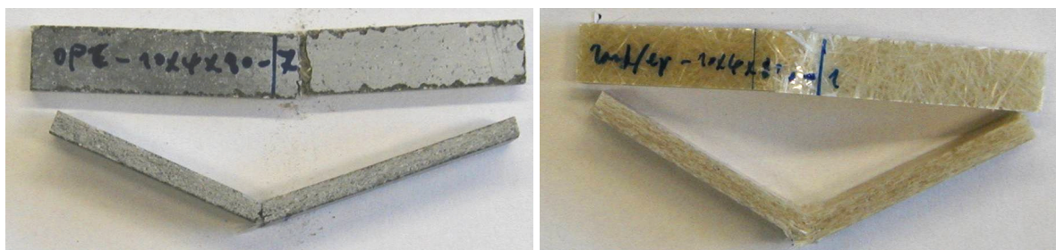
Figure 4: impacted specimens with mortar matrix (left) and epoxy matrix (right)
